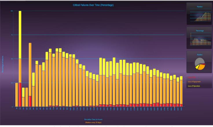
Critical Failures (Simulates the expected Critical Failures in accordance to Severity) Graph considers Replacements due to any Maintenance Activities
