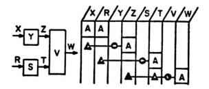
The dependency chains are arranged and grouped to form a symbolic representation of the operation of a functional group of equipment. Differences in the chains from mode to mode can also be shown. The output event specifications are then added to complete the Outline. Thus, through the use of a logical model, the complete interrelation-ship of functional elements and their associated output events is presented on the Design. Outline.
