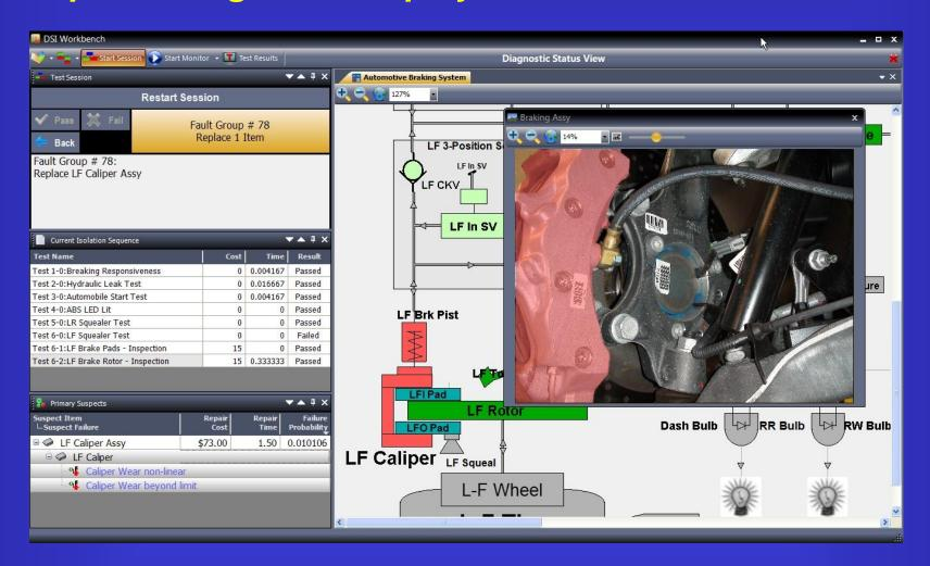
View isolated fault within DSI Workbench.
