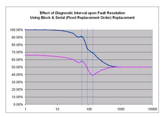
Figure 5. Effect of Diagnostic Interval upon Fault Resolution (Fixed Replacement Order)
