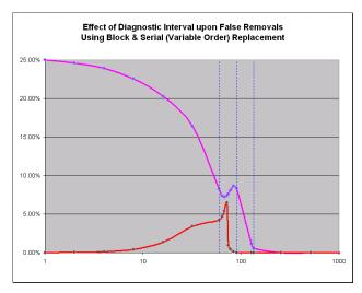
Figure 9. Effect of Diagnostic Interval upon False Removals (Variable Replacement Order)
