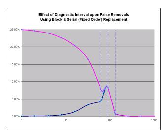
Figure 8. Effect of Diagnostic Interval upon False Removals (Fixed Replacement Order)
